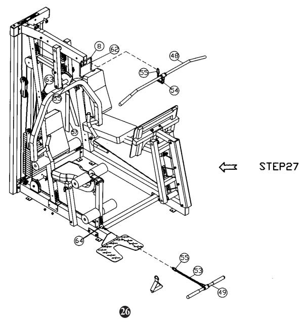
NOTE: Hand tighten bolts and nylon nuts until machine is fully assembled.
